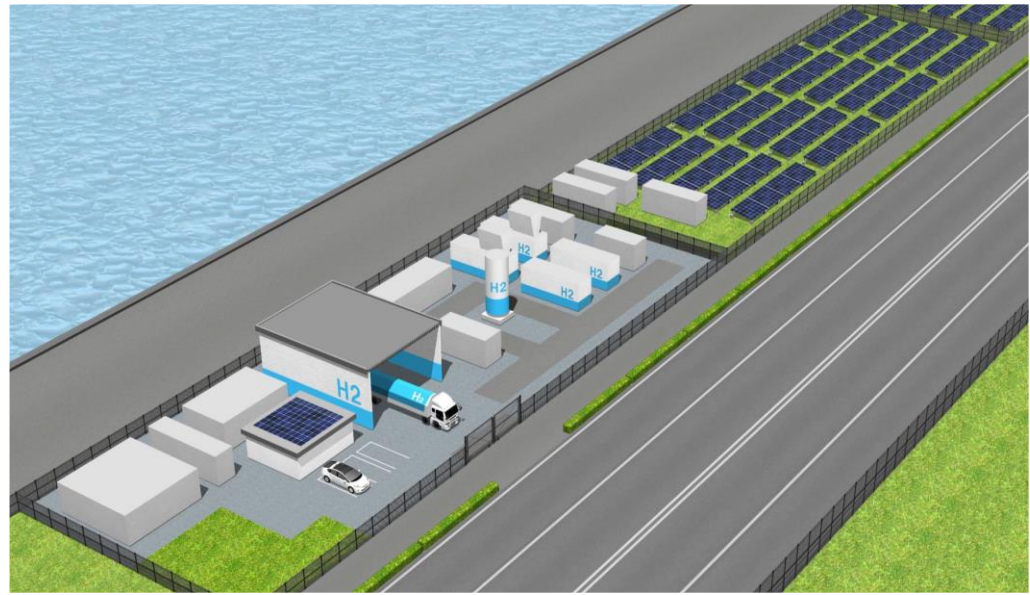
Image of the Green Hydrogen production facility at the Central Breakwater Landfill Site
