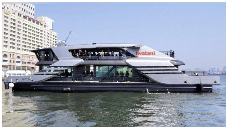
Hydrogen fuel cell ship "Mahoroba"
